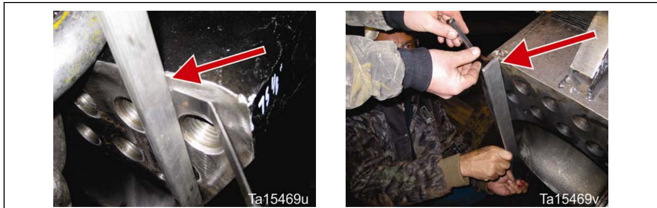
Feeler gauges under straight edge
